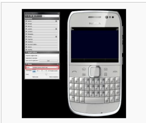
VGA resolution model in the Qt Simulator. Can be used for testing application's scalability, in special when targeting the Nokia E6 device.
