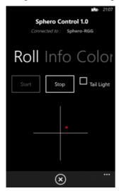
You see the red ball in the screenshot. Take a vector from (0,0) to the ball. Its angle gives the heading (0 being the Y axis) and its norm gives the speed.
