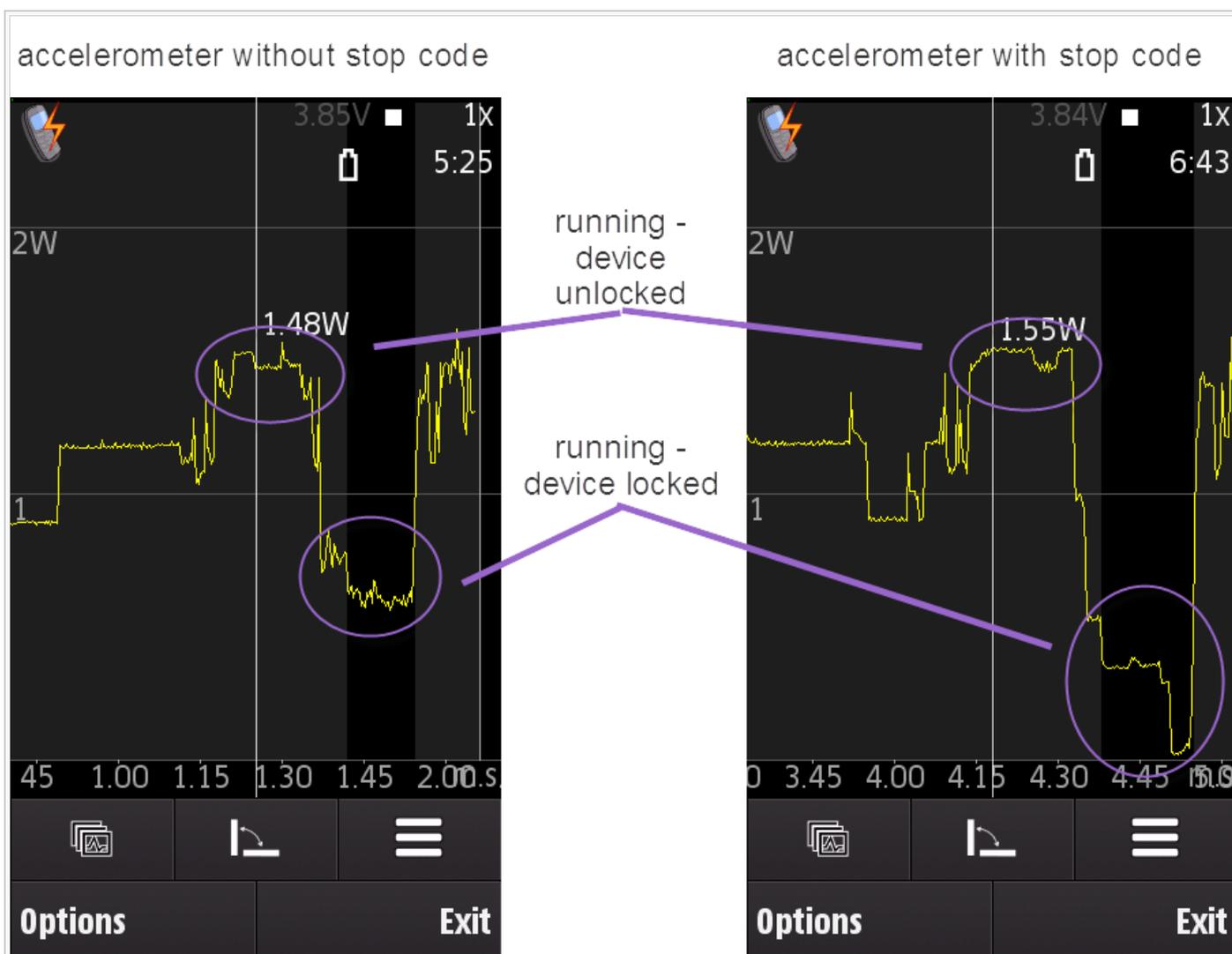
The effect on power consumption when a device is locked if the "stop" code is not included
