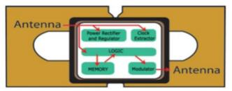
The most common of these is a "passive" tag (shown above), so-called because it has no internal battery power. Instead, passive tags are powered by energy drawn from the RF carrier wave transmitted by the reader. Following are the types of tag-
