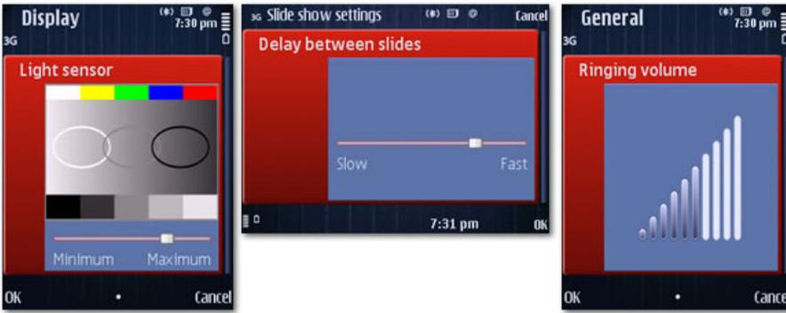
**Figure:** Various sliders in use within S60; each providing varying degrees of feedback. The ‘Ringing Volume’ control functions in a similar manner but does not provide an actual slider—only the accompanying ‘increasing scale’ visualization.
